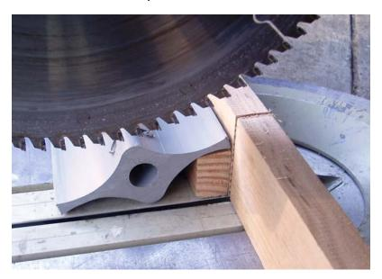
**Caution.** Tripstop must never be cut with a chain saw, a hand held portable power saw or with a blade used for ripping. If in doubt use hand operated saws. Full personal protective equipment must be worn including leather gloves, eye and hearing protective gear. A full face mask is preferable to goggles. Pieces of Tripstop less than 100 mm or 4" must never be cut using power equipment.
