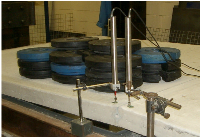
Figure 9. Slab jacked up at a corner with 200kg dead load distributed on quarter of Slab 1.
