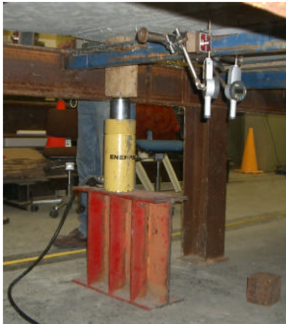
Figure 6. Slab 2 being pushed up at a corner
