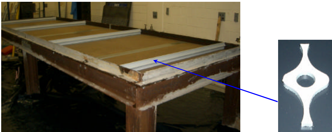
Figure 1. The locations and the cross-sectional shape of TripStop™ PVC joiners
