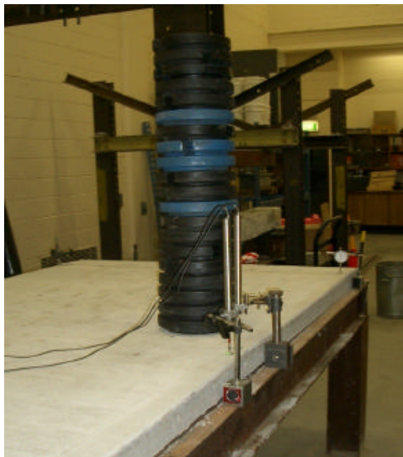
Figure 11. Slab jacked up at a corner with 200kg concentrated load applied to adjoining slab
