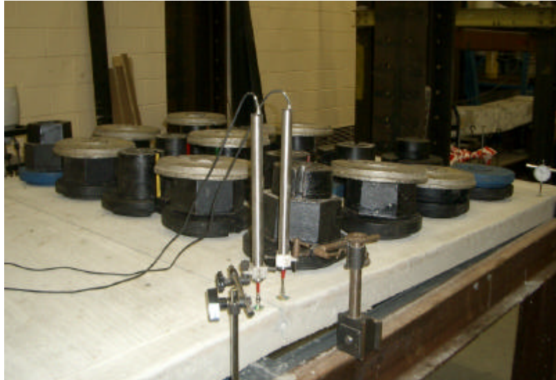
Figure 5. 490kg dead load added on the Slab 1
