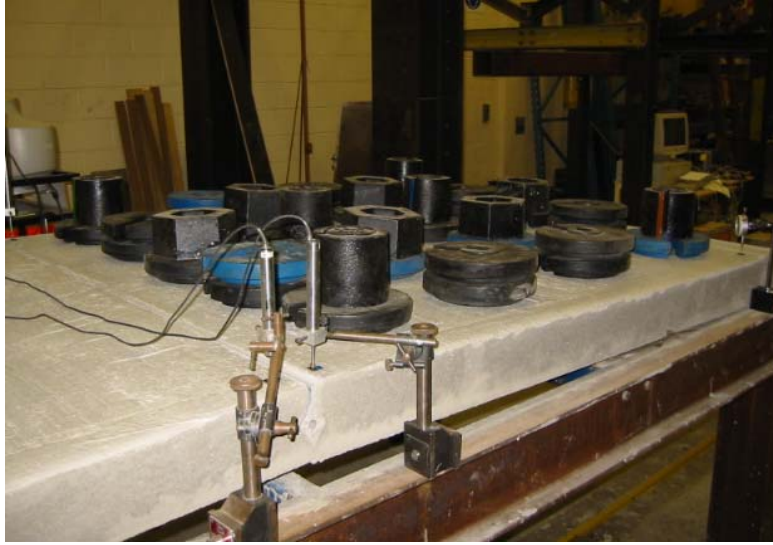
Figure 5. 400 kg dead load added on the Slab 1
