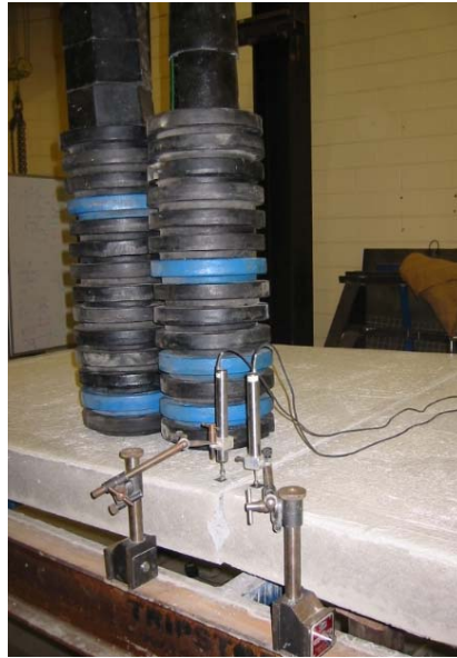
Figure 9. Slab 2 being jacked up at a corner with 400 kg concentrated load applied to adjoining slab
